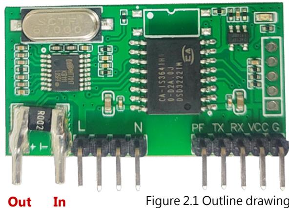
2.2.2 The live wire enters from the "IN" short end and outputs from the "OUT" end, connected to the load.
