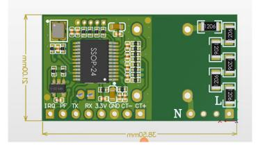
Figure 2.1 Dimensional drawing (unit: mm) Current transformer outline drawing
