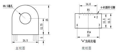
Dimensional drawing of 50A core-type current transformer
